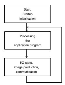
The application program is processed cyclically and can be interrupted by time- or interrupt-controlled instructions.
