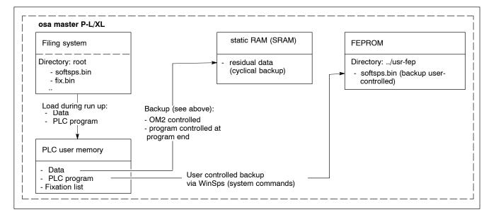
Certain residual data designated by the user are saved under program control in a special RAM area (SRAM). After the controller is switched off these data and the filing system remain in tact. On the next run up these cyclically saved data and the PLC program are available.
