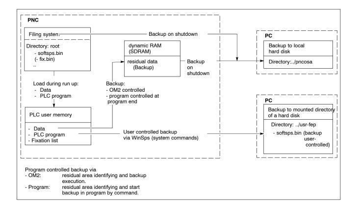
□ During normal operations the user has available the operating functions, loading and storage of the PLC program and possibly backup of the PLC project in the usr-fep directory. Cyclical backups are controlled in the OM2 or via program.
