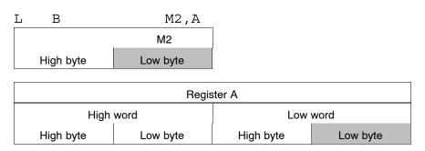
On transfer the LOW byte is addressed in the source operand (register). The destination operand may be either the even-numbered (LOW) byte or the odd-numbered (HIGH) byte.
